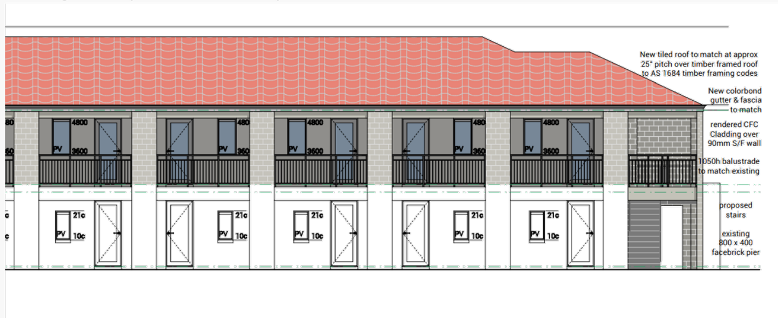
Figure 3 Upper floor extension
